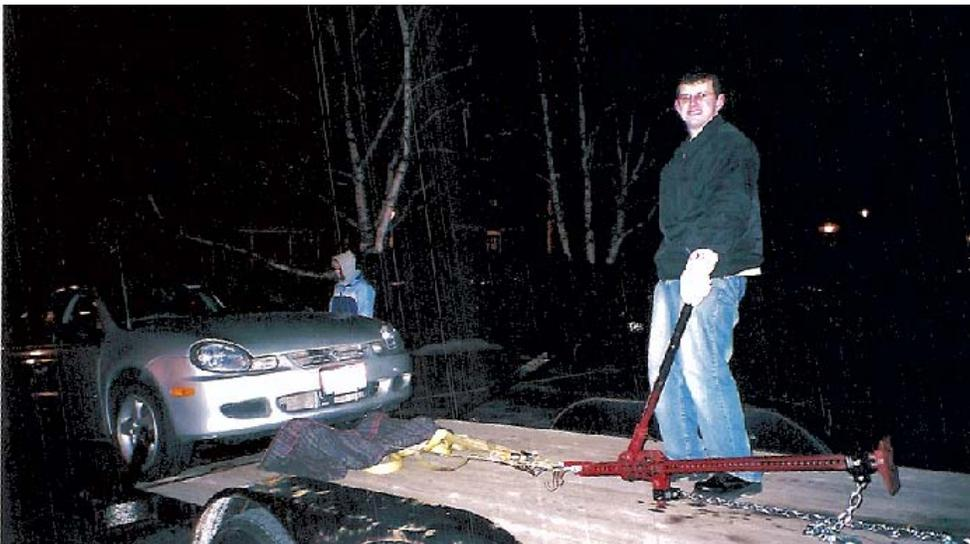
After much fiddling, we developed a system. One notch of the Hi-Lift, move up the tire chocks behind the tires. At the end of the notches, set the parking brake, adjust the chain, take off the parking brake (an important step only forgotten once) and start again. When the chain ran out, adjusted the ratchet straps. And when the ratchet straps were too short, the car was up onto the trailer (finally!) and only a small shove to the center of the trailer. And
